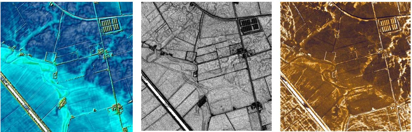
Fig. A3.3 River Witham: : left, relief-shaded colour scale; centre, sky-view factor; right, total insolation
